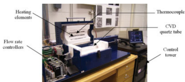
Figure 1. Easytube 1000 CVD (first nano) system at the Clemson University Smart Structures and Nanoelectromechanical Systems (SSNEMS) Laboratory.
